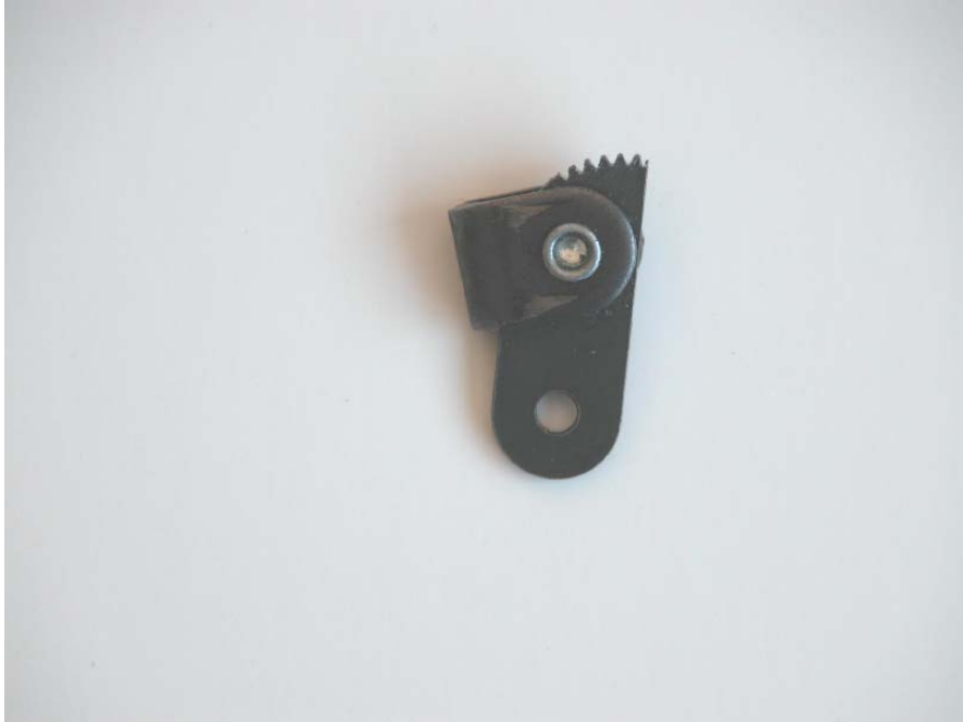
Figure 2. Lock-Cam – 116BS cam lock (Halford Hide and Leather Co., Edmonton, AB Canada) with filed gripping teeth used to test breakaway snares near Vegreville, Alberta, Canada, during 2004-05.
