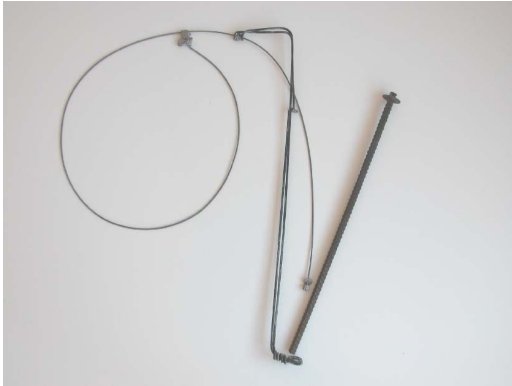
Figure 1. Grawe's snare support system used to test breakaway snares near Vegreville, Alberta, Canada, during 2004-05.
